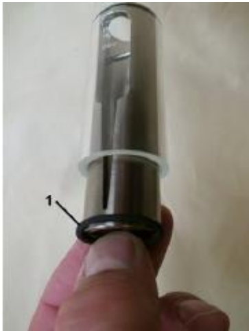
Fig. 47: Centering the slot nozzle
