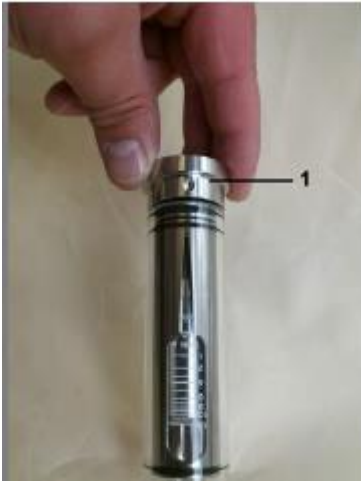
Fig. 49: Process connection (Inlet)
