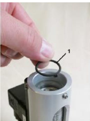
Fig. 54: O-ring, slot nozzle buffer
