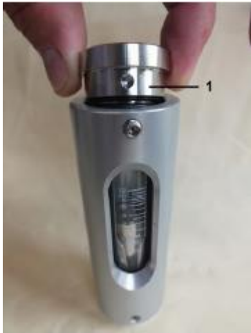
Fig. 55: Position the outlet process connection
