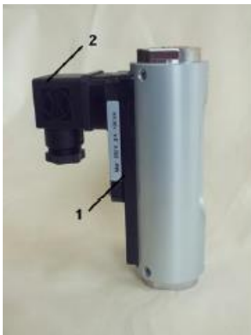
Fig. 3: Switch contact and female socket A potential-free Reed-contact is cast into the switch contact housing assembly. ( Fig. 3/1). The device is supplied with a connector Fig. 3/2).
