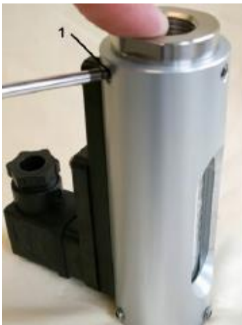
Fig. 52: Secure the process connection (inlet)
