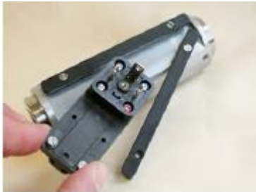
Fig. 63: Remove switch contact
