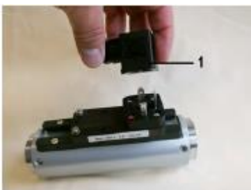
Fig. 59: Remove the female socket
