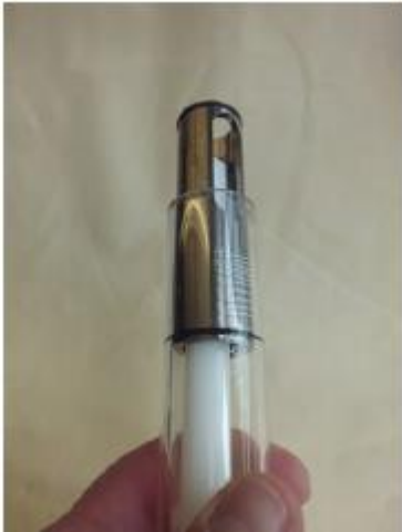
Fig. 41: Remove slot nozzle
