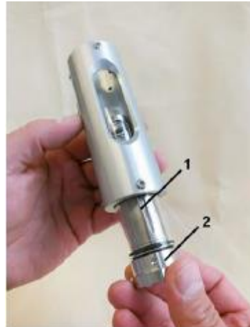
Fig. 40: Remove the inner section
