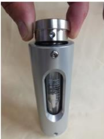
Fig. 37: Remove the process connection (outlet)
