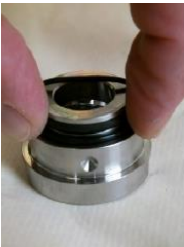
Fig. 43: O-ring (glass buffer)
