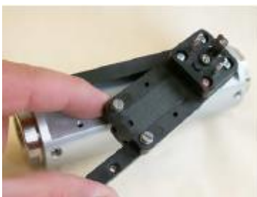
Fig. 62: Rotate guide rail to the side
