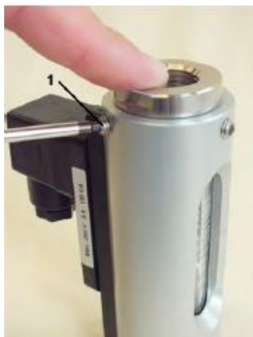
Fig. 56: Tighten hex socket screws
