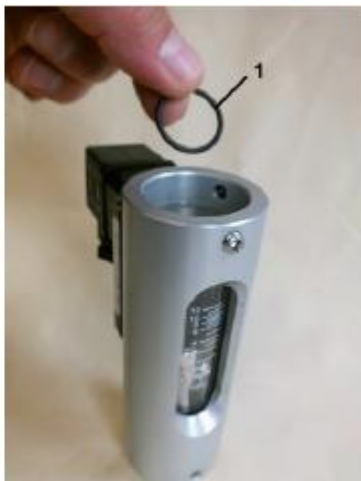
Fig. 37: Remove the process connection (outlet)
