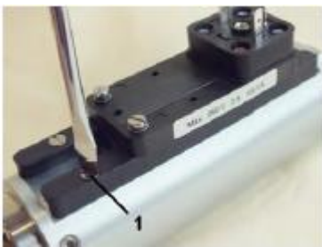
Fig. 61: Release the guide rail
