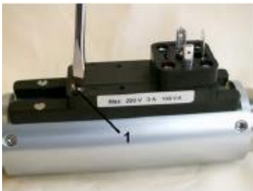
Fig. 60: Loosen set screws
