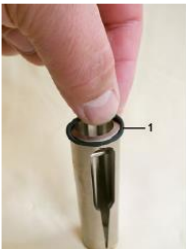
Fig. 45: O-ring (centering the slot nozzle)
